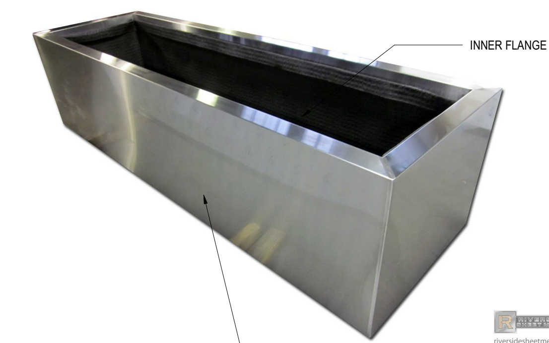
18 GA BRUSHED STAINLESS STEEL #4 FINISH PLANTERS PROVIDED BY OWNER AND ARE TO MATCH EXISTING RAILING AT FRONT RAMP. PROVIDE 3" BASE TO MATCH MANUFACTURER TO PROVIDE LEVELING AND WEeping DETAILS.
